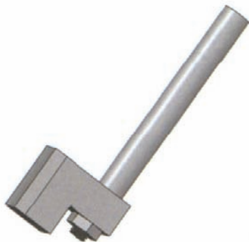
图1 成型电极 Fig.1 Forming electrode
